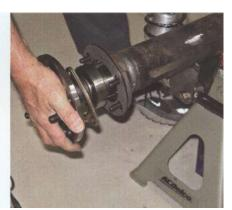
1. Installation must begin by taking the axles out of the housing. Start by installing the t-bolts into the housing flange. The spacer plate can then be installed on the end
