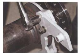
7. Remove rotor and bolt the caliper bracket to the base bracket using the spacer(s) determined in the previous step.
