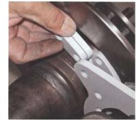
6. Test fit the caliper on the rotor, making sure the bleed screw is facing up. Your brake kit comes with bracket spacers in two different thicknesses. Determine the number and thickness of spacers required to properly position the caliper in relation to the rotor.
