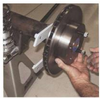
8. Re-install rotor, again using two lug nuts to hold it in place.
