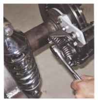
9. Install caliper on bracket using supplied Allen-head slider bolts.
