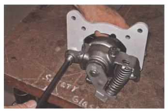
5. Insert the brake pads in the caliper and install the caliper brackets as shown using the supplied Allen-head slider bolts.
