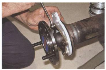
2. Install the base bracket between the spacer and the retainer and secure using the supplied nuts. The ears on the base bracket should be positioned so they will mount the caliper up toward the rear as shown.
