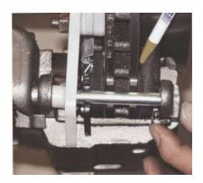
10. With caliper installed, double check to verify the gap between the brake pads and rotors is equal on both sides. Adjust shim packs as needed to achieve equal gap.
