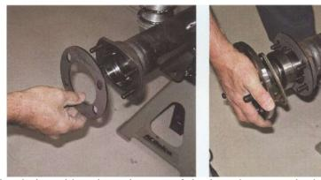
1.Installation must begin by taking the axles out of the housing. Start by installing the t-bolts into the housing flange. The spacer plate can then be installed on the end
