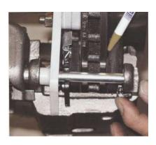
10. With caliper installed, double check to verify the gap between the brake pads and rotors is equal on both sides. Adjust shim packs as needed to achieve equal gap.
