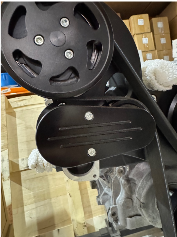
Figure 6. Belt tensioner front cover installed.
