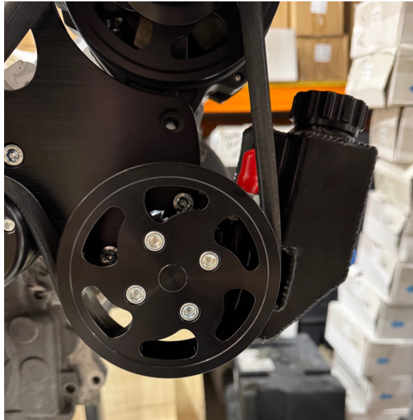
Figure 4. Power steering pump installation through pulley cut-outs.
