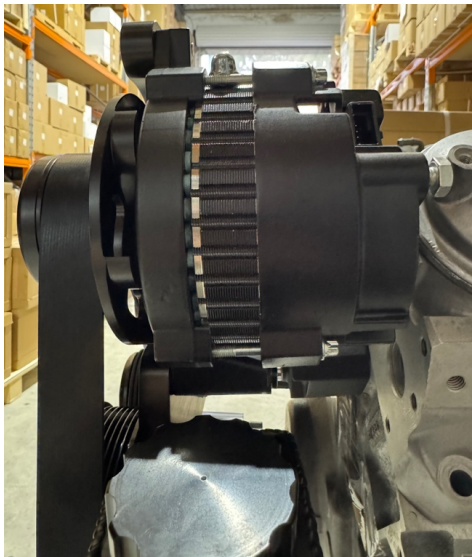
Figure 3. Alternator installation orientation.
